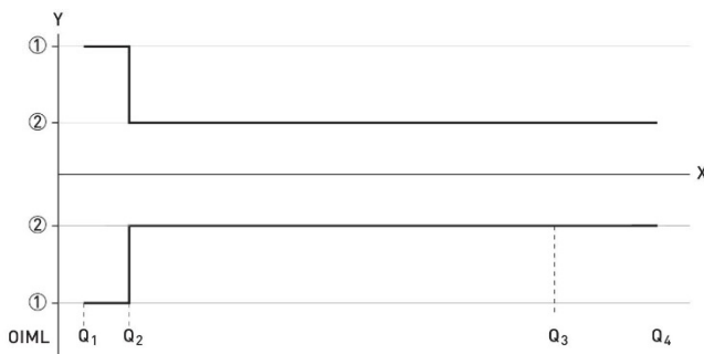
Figure 2-1: ISO flow rates added to figure as comparison towards OIML X: Flow rate Y [%]: Maximum measuring error ① ± 3% for class 1, ± 5% for class 2 devices ② ± 1% for class 1, ± 2% for class 2 devices
